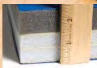
1" POLYFOAM LAYER AND A FIRMER 1 3/8" POLYETHYLENE LAYER
